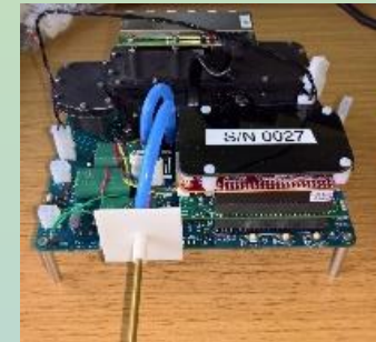
POPS (Handix Scientific company, USA) 1 kg payload
