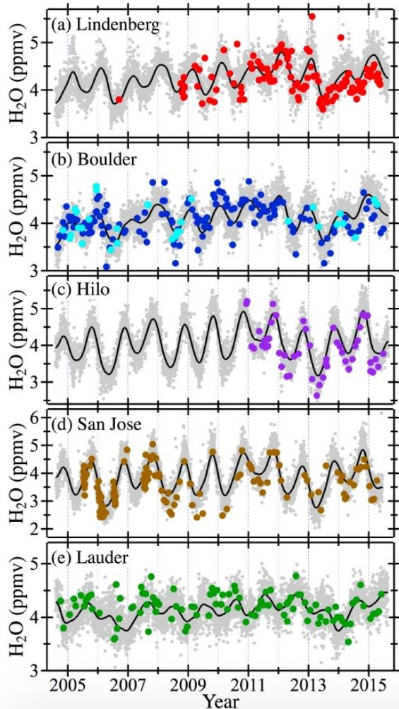
Daily MLS H<sub>2</sub>O, reference satellite data, vs. in situ frost point hygrometer data at 68 hPa (filled circles).
