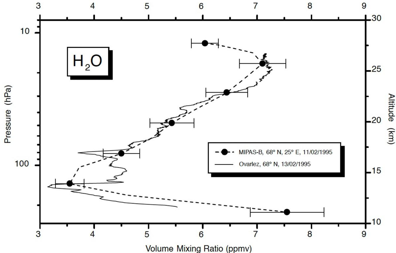
Balloon-borne frost-point hygrometer and MIPAS satellite measurements of H<sub>2</sub>O profiles inside the Arctic vortex in Feb. 1995 [SPARC, 2000]
