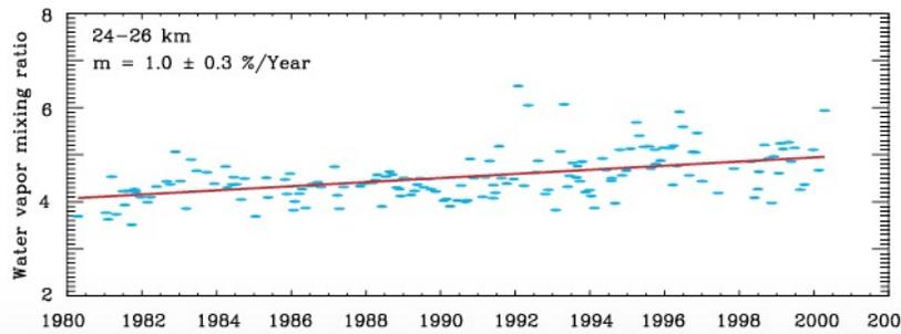
Time series of 2 km layer average H<sub>2</sub>O (in ppmv) over Boulder. Data from balloon-borne frost point hygrometers [SPARC, 2000].
