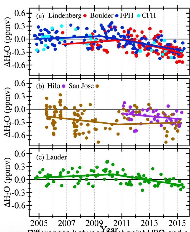
Differences between frost point H<sub>2</sub>O and coincident MLS H<sub>2</sub>O over the five sounding sites. Two distinct periods separated by a changepoint [Hurst et al., 2016]
