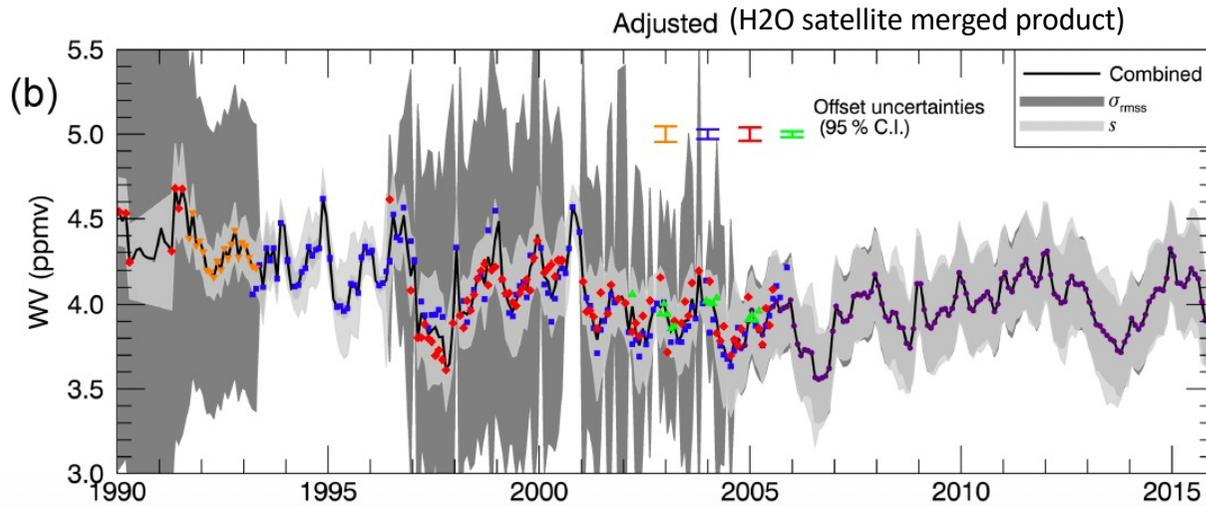
(a) Top: Uncorrected satellite H<sub>2</sub>O time series in 30-40S band at 68 hPa (~18 km), (b) Bottom: Offset-corrected satellite series [Davis et al., 2016]
