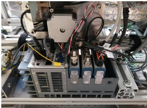
**cRIO 9031 (National Instruments) controller:** 1.33GHz, 1GB RAM, x2 serial, x2 RS485, x2 Ethernet ports, -40 °C to +70 °C
