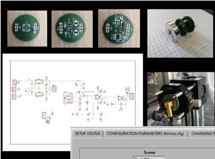
New miniaturized PCB for pyroelectric detectors (designed by CNR-INO electronics workshop)
