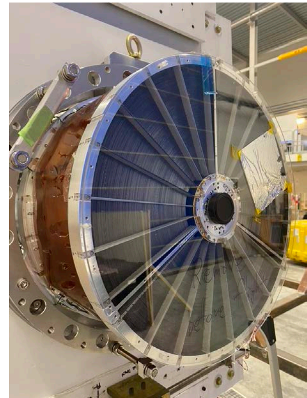
X-ray mirror (Hitomi spare) 213 nested Pt/C-coated shells (Wolter I) Effective area: 180 cm 2 @ 30 keV
