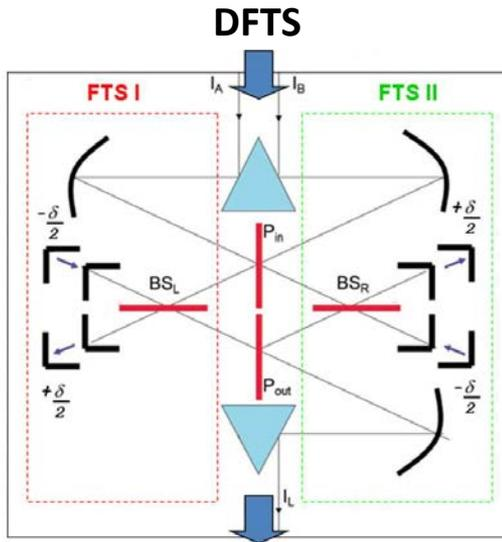
**spectrometer on chip** (in one of the 4 channels):
