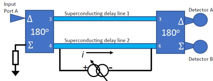
Two superconducting delay lines:
