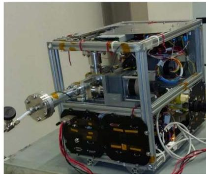
The particles are collected in a ultra high vacuum collecting chamber. The experiment is designed to have very low particles contamination.
