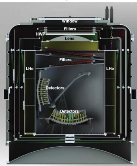
**Cryogenic system** : vacuum shell,
