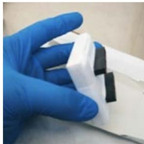
Gagg scintillator optically coupled to a single large sensitive area SiPM (Silicon Photo Multiplier) array
