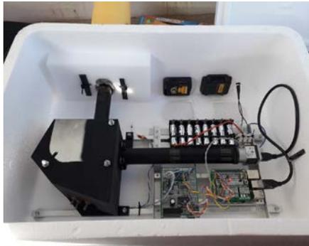
Tecnological flight: Demonstration of a static Fourier Spectrometer, in the optical and IF bands, that uses Littrow prisms as dispersive elements. The instrument has high signal to noise ratio and high luminosity
