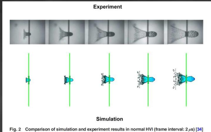
Fig. 2 Comparison of simulation and experiment results in normal HVI (frame interval: 2  $\mu$ s) [34]
