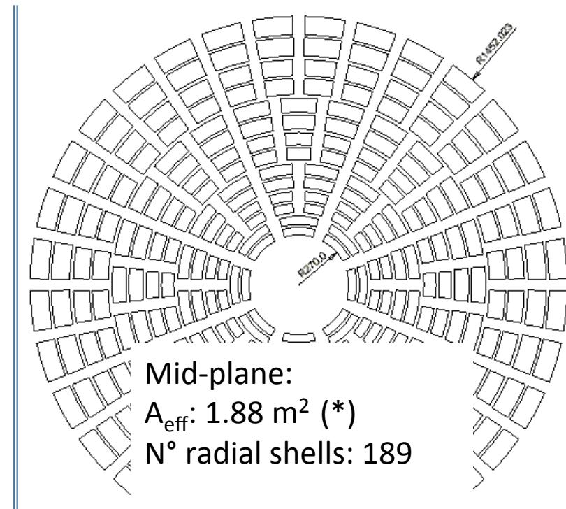
(\*) @ 1keV with 30' off-axis angle for shell spacing and without ribs (oscurring 5 %)
