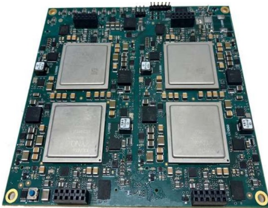
The ExaNeSt Quad-FPGA Daughter Board (QFDB).
