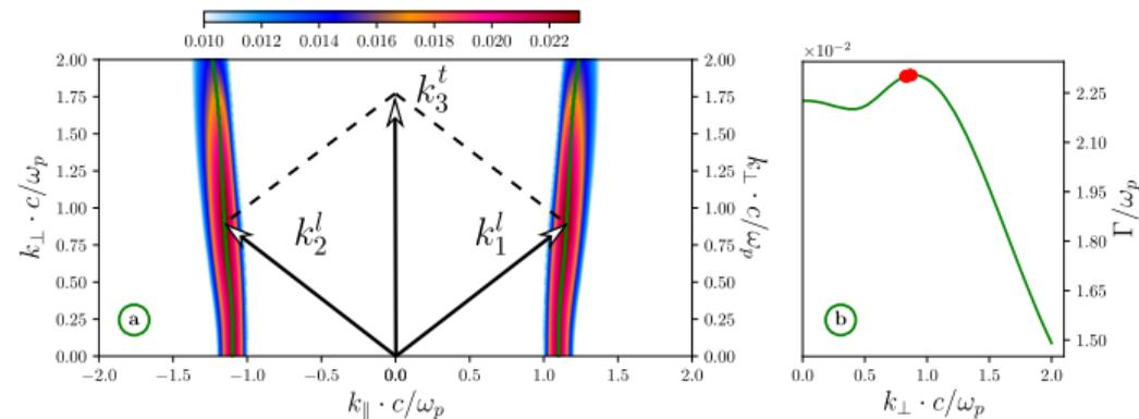
(a) The growth rate map for the beam-plasma instability  $\Gamma(k_{\parallel}, k_{\perp})$  in the efficient regime. The green line  $k_{\perp} = k_{\perp}(k_{\parallel})$  mark the maximal growth rate achieved for each  $k_{\perp}$ . (b)  $\Gamma(k_{\perp})$  along the green line (red points indicates the region of the three-wave interaction).
