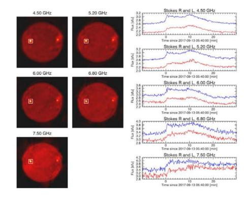
Radio images of the Sun (left) from SRH for September 13, 2017. The active region in which the jet was observed is marked with a white rectangle. Microwave flux light curves for this region in the right (RCP, blue) and left (LCP, red) polarization are shown in the right panels
