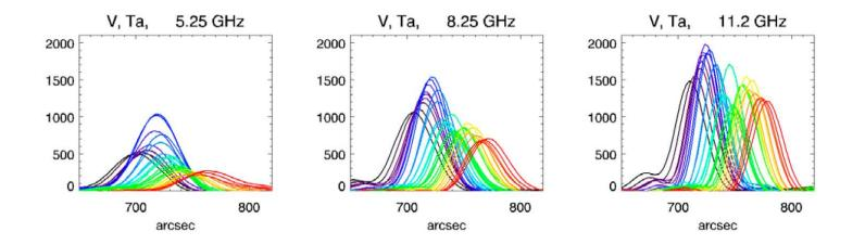
RATAN-600 scans of antenna temperatures of polarized radiation in AR 12738 on April 17, 2019 at frequencies of 5.25, 8.25, and 11.20 GHz. Different colors indicate observations in different azimuths: 31 records in a time span 07:11–11:15 UT with a step of 8 min. The left-to-right shift of the scans is a projection effect associated with the Earth rotation and depending on the orientation of a radio telescope antenna. Jet passage time corresponds to a radiation increase in blue scans
