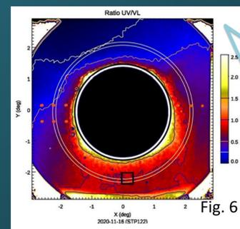
**Working hypothesis:** Assuming that at each point of the door the reflectance ratio for the 2 channels is the same, we can try to use UV2VL ratio to correct the data.
