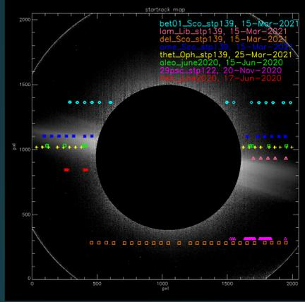
This map shows the tracks of the stars analysed up to now, in the Field of View (FoV) of the Metis VL channel. While the stellar target opportunity is very rich for the VL channel, it is important to consider that the available targets for the UV channel are relevantly less and this constraint was fundamental in the planning of the stellar observations, as they prioritized the few available targets falling within the Metis FoV.
