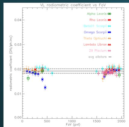
In this plot the first results of the data inversion: the value of the radiometric coefficient (in DN per incident photon on the instrument aperture) vs the FoV position for different stars. The values are consistent between the several stars. This analysis provides the radiometric coefficient to pass from L0 data (in digital units) to L2 data (in physical units).
