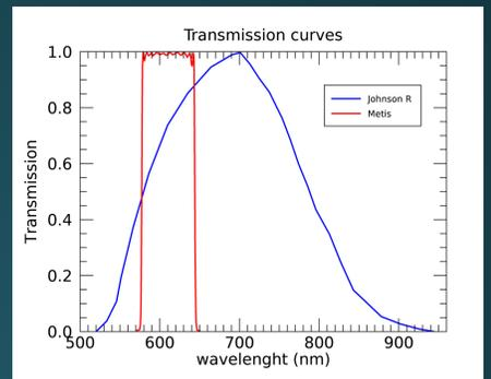
Fig. 4: Comparison between the transmission curves of the Metis VL filter and Johnson standard red filter.
