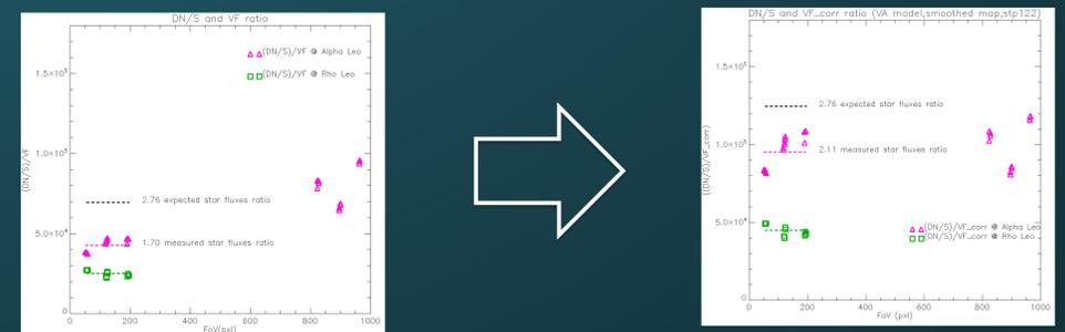
Fig. 7 – Left panel: Counts per second divided by the VF along the FoV, for  $\alpha$  and  $\rho$  Leonis. Right panel: Same ratio of the left panel “corrected” with the UV2VL ratio map.
