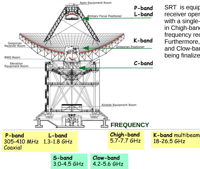
SRT is equipped with a 7-beam receiver operating in K-band, with a single-beam receiver in Chigh-band, and with a dual frequency receiver in P/L band. Furthermore, two new S-band and Clow-band receivers are being finalized.
