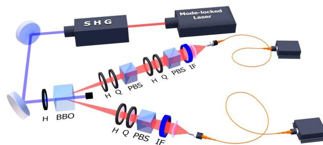
SHG: Second-harmonic generation; BBO:  $\beta$ -barium borate crystal; H: half-wave plate; Q: quarter-wave plate; PBS: polarising beam splitter; IF: interference filter.
