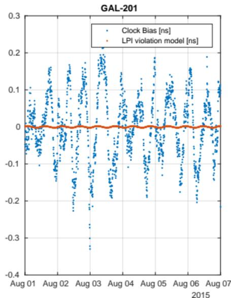
Fit of the LPI violation model with **Linear Least Square** in a **Monte Carlo routine**: 1 GR violation parameter ( $\alpha$ ) + 2 parameters per day fitted (daily clock offset  $a_i$  and drift  $b_i$ )
