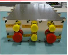
Stack Current Source and Impedance Measurement Unit (SCS IMU)
