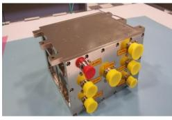
CO2 Reprocessing Assembly Power Supply Module (CRA PSM)
