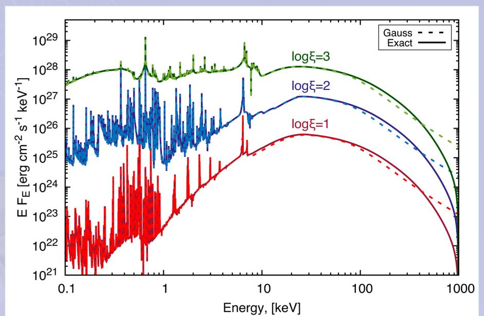
Full calculations of reflected spectra with the XILLVER code, including all relevant atomic transitions, for a slab at constant density ( $n_e=10^{15} \text{ cm}^{-3}$ ) for 3 different ionization parameter  $\xi = 4\pi F_X/n_e = 10, 100, 1000 \text{ erg cm}^2 \text{ s}$ . Compton scattering inside the slab is calculated with the traditional Gaussian approximation for the energy redistribution of photons (dashed lines), and with the exact solution from Nagirner & Poutanen (1993).
