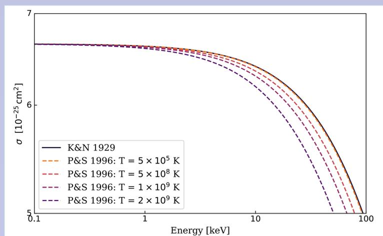
Comparison of the total quantum electrodynamic cross section for Compton scattering of photons off stationary electrons (Klein & Nishina, 1929), and the Klein-Nishina cross section convolved with a relativistic Maxwellian (Poutanen & Svensson, 1996). As expected, the largest departures occur at high electron temperatures.
