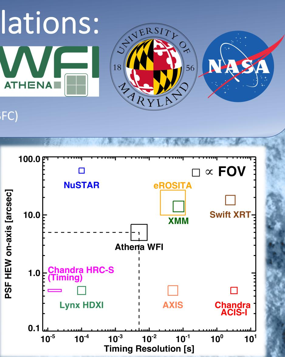
The Athena wide-field imager (WFI) will be a time domain survey machine in the X-ray band. Athena WFI will have an ideal combination of angular/timing resolution, field of view, and sensitivity to revolutionize the study of accreting black hole and neutron star systems (observed as X-ray binaries).
