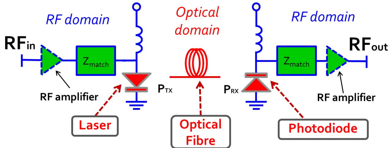
Cheaper, lighter, smaller than copper cables
