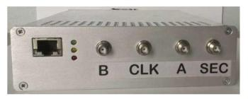
Fig. 9. Front view of the ADR box, that contains the boards displayed in Fig. 8. The input labels correspond to those of Fig. 6 (with for A = input 1 and B = input 2). The receiver can operate independently in a section of the radio telescope or installed in the ADR Server).
