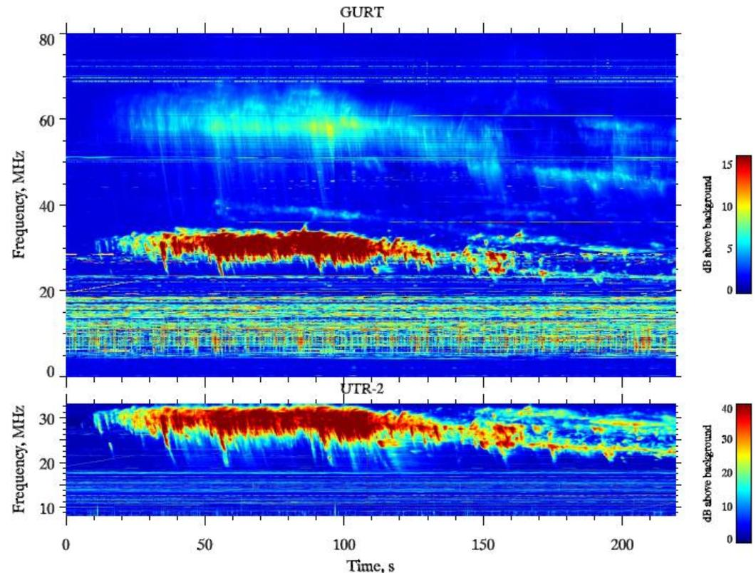
Fig. 10. Observations of a type II burst. UTR-2 frequency band 8.25 ÷ 33 MHz frequency and time resolution of 4 kHz and 100 ms, respectively. Recording was conducted on subarray GURT in the range 8 ÷ 80 MHz with the same time resolution and frequency resolution of 20 kHz. Start recording corresponds to 07:11:15 UT.
