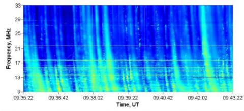
Fig. 7 Dynamic spectrum with a sequence of solar bursts of type III and IIIb-III obtained by the DSPZ connected to the South arm of UTR-2 on July 8, 2014
