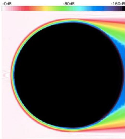
Attenuation of a 60 kHz radio wave due to propagation around the Moon with subsurface penetration and a lunar density model (Takahashi, 2003)
