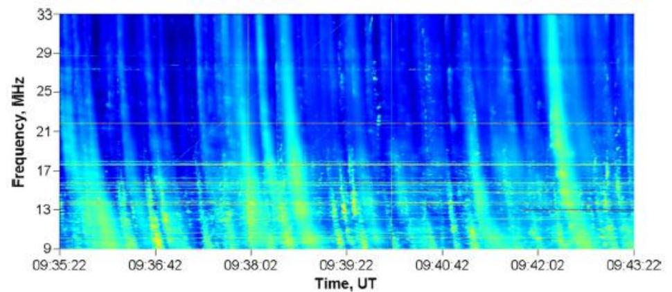
Fig. 7 Dynamic spectrum with a sequence of solar bursts of type III and IIIb-III obtained by the DSPZ connected to the South arm of UTR-2 on July 8, 2014
