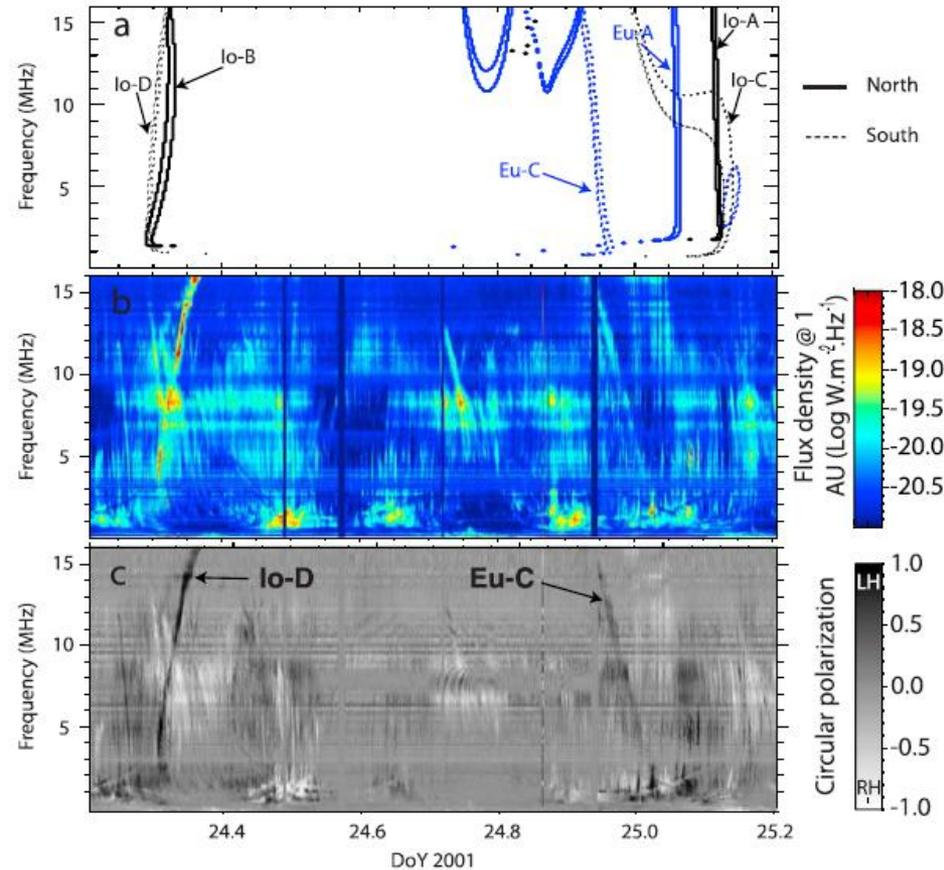
**Figure 2.** Cassini observations of an Io and a Europa arc. (a) EXPRES simulations (Io in black and Europa in blue—thick line, northern emissions; dotted line, southern emissions), (b) Intensity flux and (c) the circular polarization—LH: left handed (emission from the southern hemisphere); RH: right handed (emission from the northern hemisphere). This time interval was chosen because of the presence of an Io arc and a Europa arc.
