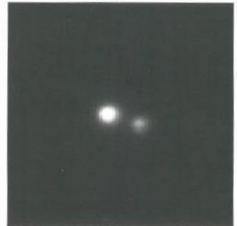
Fig. 7.2 - The first object observed: epsilon-lirae double-star system, separation: 2.6", profile FWHM: 0.8"
