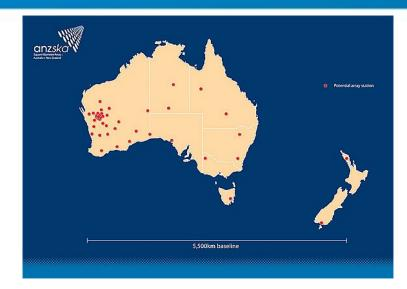
SKA Low, in Australia 256000 antennae Randomly placed Band 50-350Mhz
