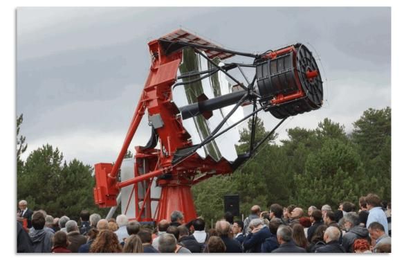
The ASTRI SST-2M telescope works like every IACT telescope by imaging the very short flash of Cherenkov radiation generated by the cascade of relativistic charged particles produced when a very-high-energy gamma-ray strikes the atmosphere. The collecting mirror system reflects the Cherenkov light to a high-speed camera that digitizes and records the image of the shower.
