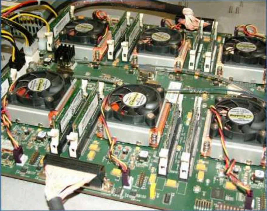
e.g. FPGAs in the ASKAP correlator
