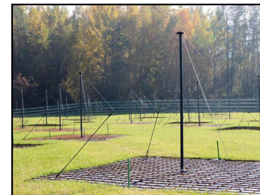
Low-band antennas 10-90 MHz
