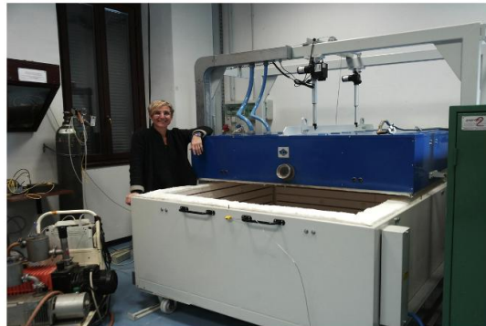
Oven for hot forming of thin glass foils
