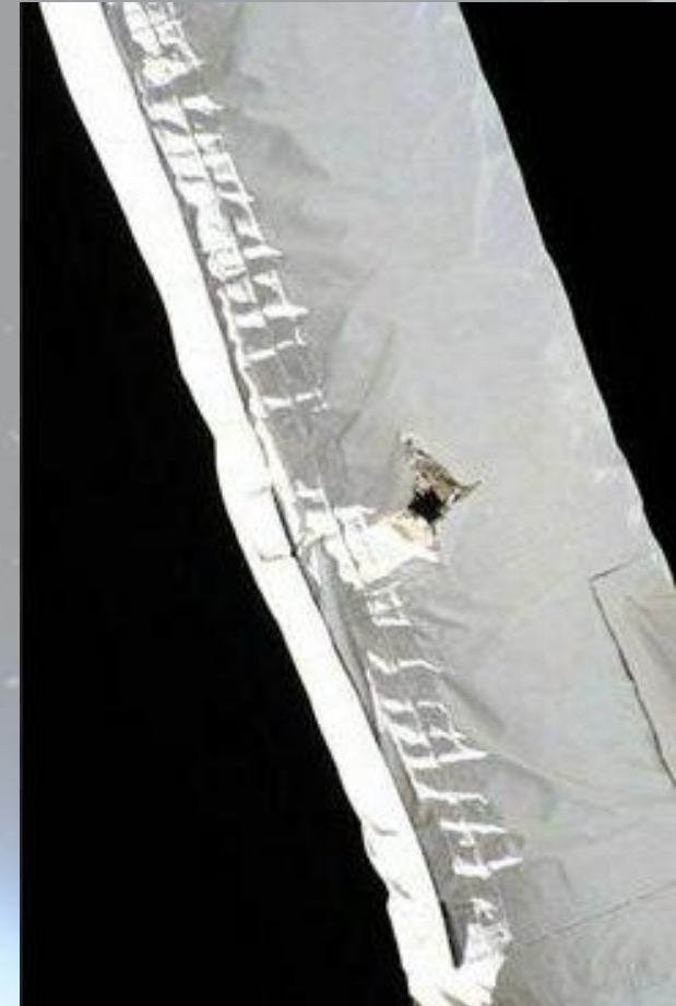
Effect of a microimpact on a robotic arm of the ISS.
