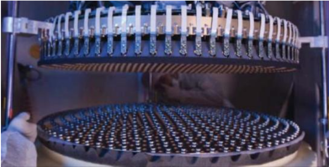
LBT Gregorian Secondary Mirror with 672 actuators
