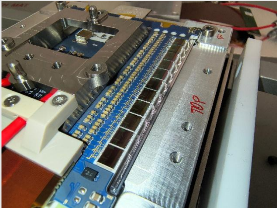
Detector Assembly: sensor side (top), ASIC side (bottom)
