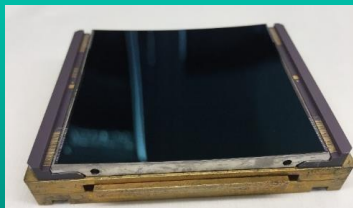
Curved-silicon 2D array CCD with 500 mm radius
