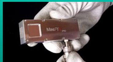
GaAs on MiniPix TPX3 for high energy detection
