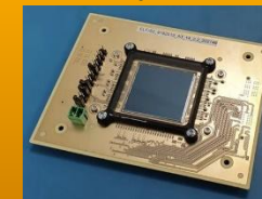
ELFIS II: Low flux CMOS sensor from a European supply-chain
