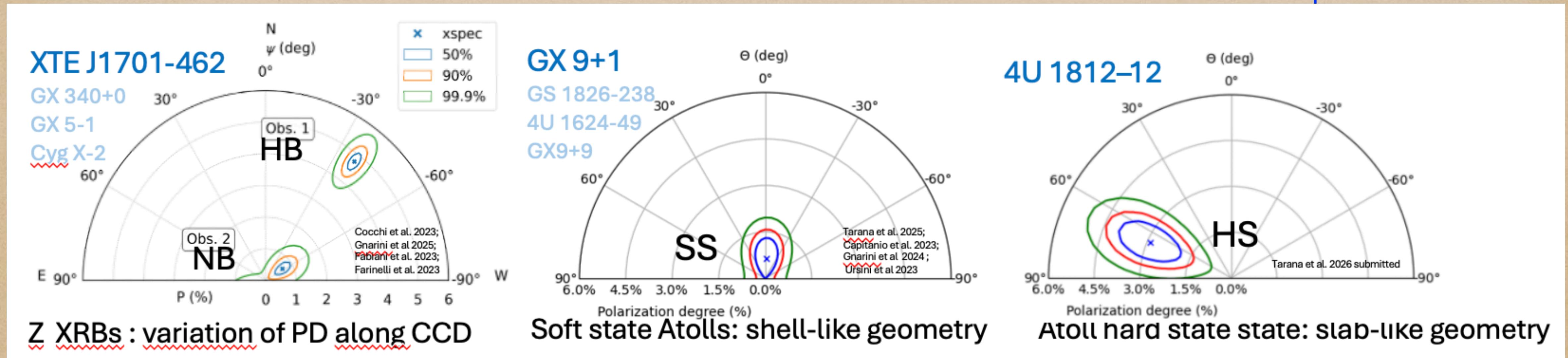
Geometry of accretion flow changes with source spectral state
