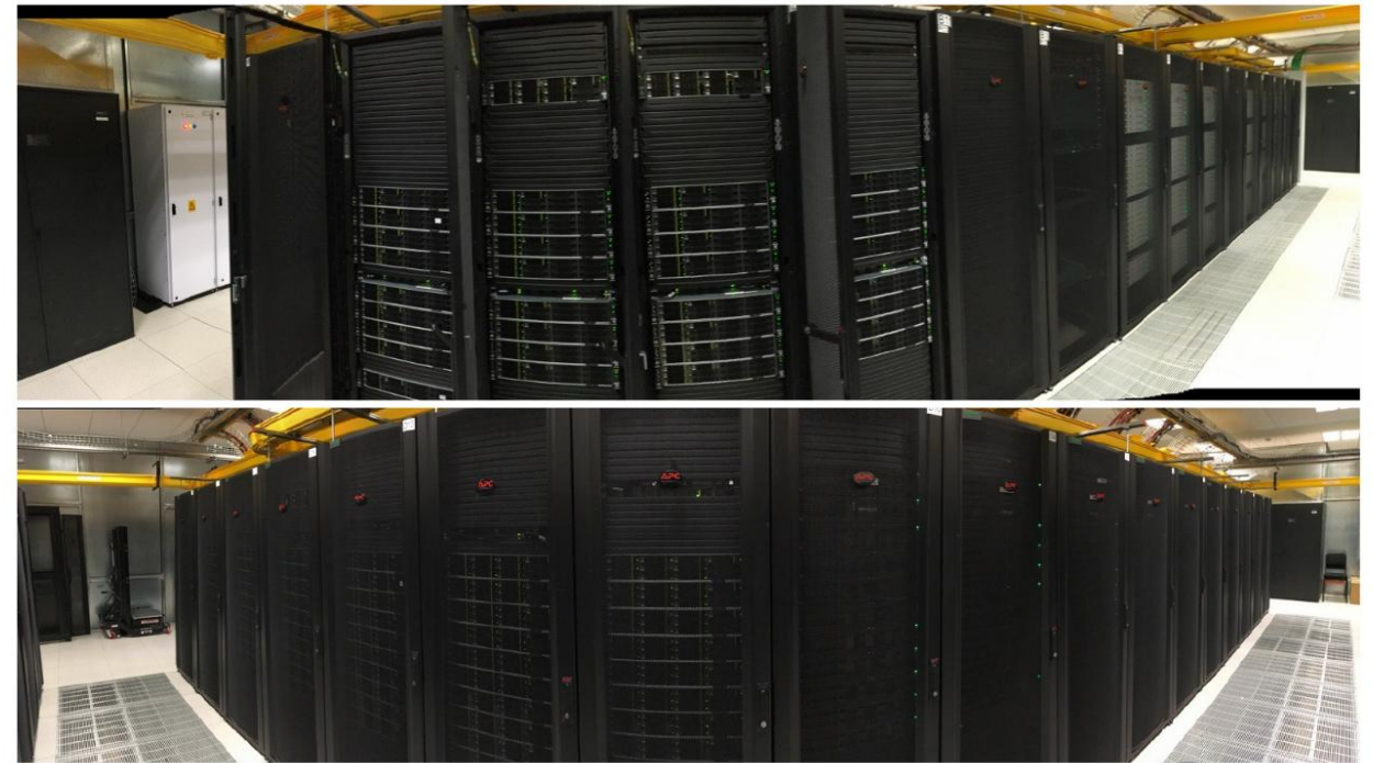
Figure 3.2: A fish-eye view of the TRAPUM user supplied equipment (USE) at the KAPB. Top panel is the FBFUSE rack. Bottom panel shows APSUSE consisting of 7 racks from the left with the rest belonging to TUSE. (Credits: E. Barr)
