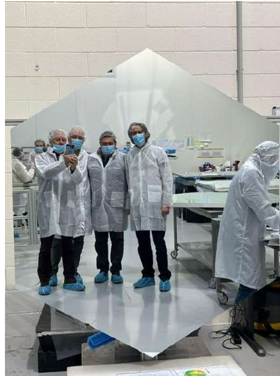
Cherenkov LST/CTAO mirror (core of Al hexacell)
