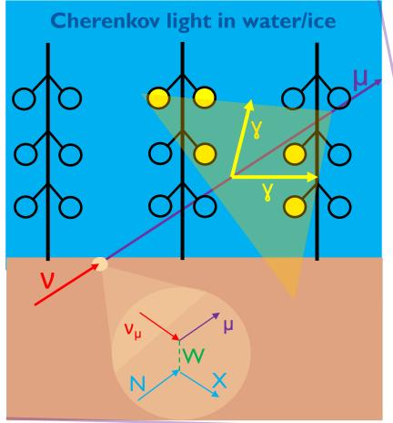
Cherenkov radiation detected by arrays of PMTs
