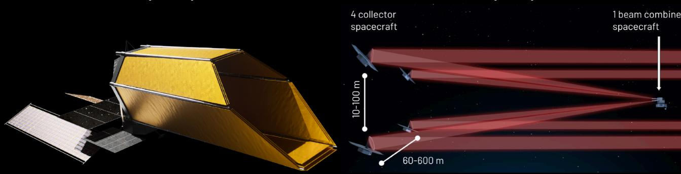
6-8m mirror Coronograph w/  $10^{-10}$  contrast Reflected light 0.2-1.8 µm, R = 70-200 4 mirrors (2.0-3.5m) Nulling interferometry Thermal emission 6-16  $\mu$ m (4-18.5  $\mu$ m goal), R = 100
