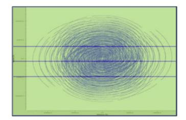
Grid **unequally distributed** among processing units – **balanced** gridding, but unbalanced FFT
