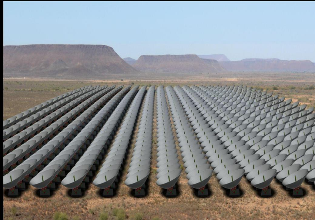
**HIRAX** is **radio telescope** array that will map nearly all of the **southern sky** in **radio continuum** and **neutral hydrogen line emission** over a frequency range of **400 - 800MHz**
