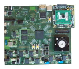
12Gs/s ADC FPGA board for radar system (Italian Navy)
