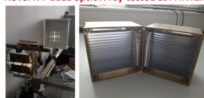
Novel K-P Baez optic X-ray tested at PANTER
