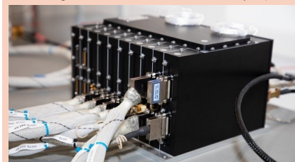
Photo of the flight model of the onboard ECLAIRs management and scientific processing unit (UGTS, unité de gestion et de traitements scientifiques)
