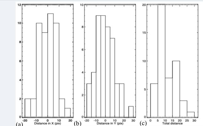
Figure 6: The distance (in pixels/arcsec) between predicted and measured ghost positions as histograms in (a) X, (b) Y and (c) total.
