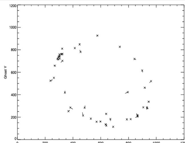
Figure 5: Ghost positions (crosses), with a line indicating the shift between the actual and predicted positions, showing there is no particular pattern to the error scatter.
