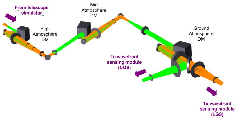
Turbulence can also be injected via DM commands!
