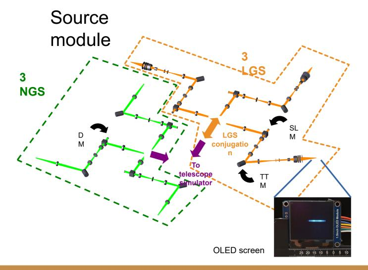
**3 NGSs** and **3 LGSs** (the latter simulated with OLED screens to reproduce the source elongation)
