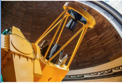
Figure 1. The 1.65-meter Ritchey-Chrétien telescope used to observe the stars analyzed in this study.
