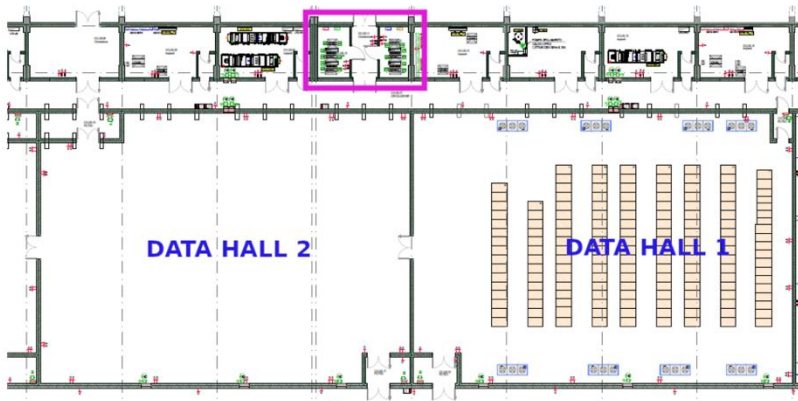
Figure 2. Technopole data centre floor plan. Leonardo layout is depicted in Data Hall 1 (on the right) and the procured System will be hosted in Data Hall 2 (on the left). The network room is indicated by a purple box at the top of the figure.
