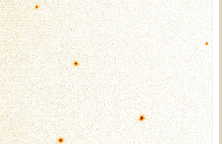
RESULTS: we used an EO-5012M CMOS camera (pix size: 2.2 x 2.2  $\mu$ m; 2560x1920 pix). Left panel shows a laboratory stellar field in white light of 5° x 5°. Right panel shows a single source with horizontal and vertical graphs. FWHM is around 6 x 6 pixels, in good agreement with the design.
