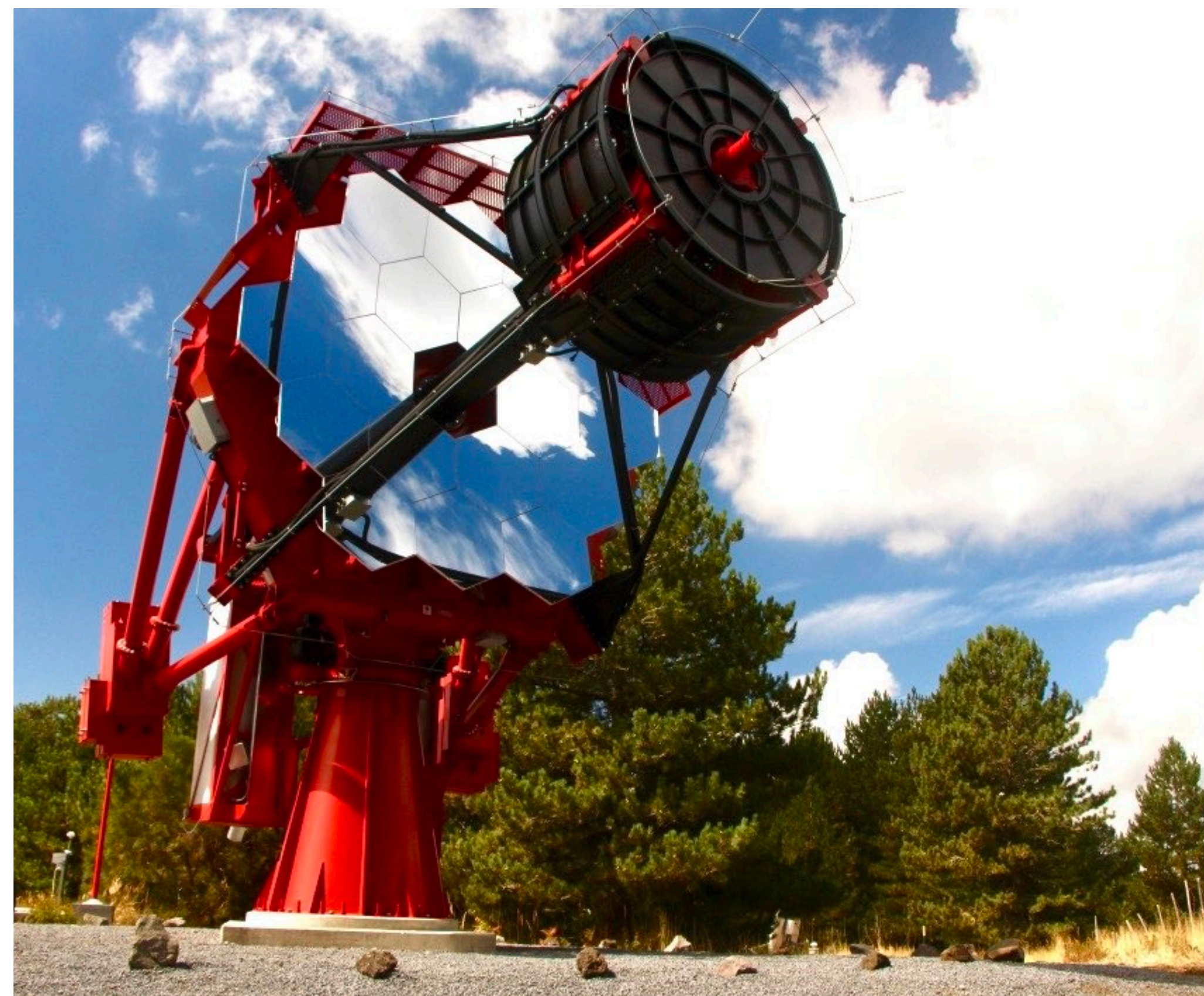
Fig. 1: The prototype telescope ASTRI-Horn [2], on Mount Etna. It is an example of Imaging Atmospheric Cherenkov Telescope [3] and its mirrors suffer from fast degradation due to gases and dust released during eruptions of volcano.
