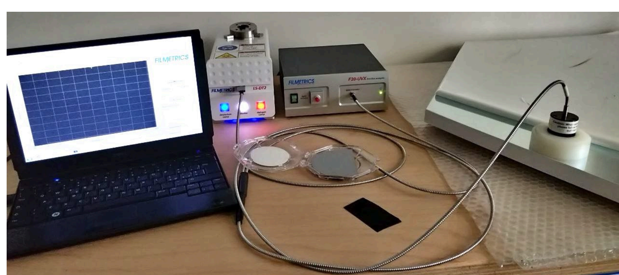
Fig. 2: Experimental setup for reflectivity measurements in lab.
