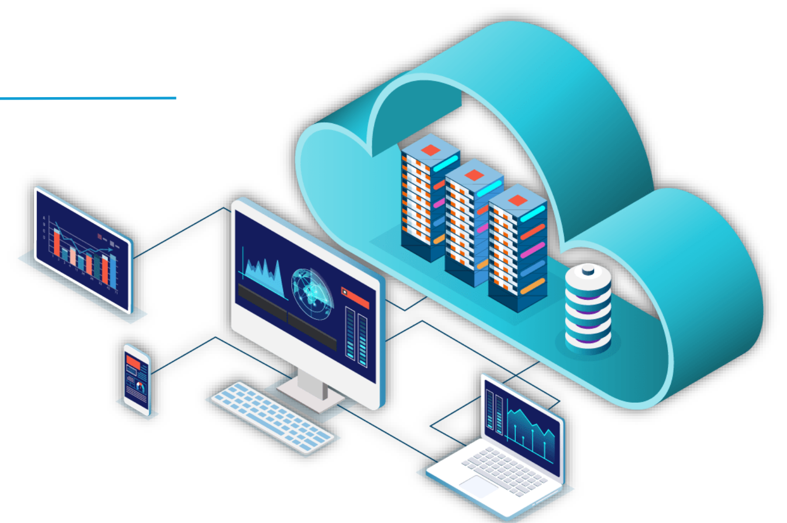
Fig. 4 – The HyperLab system utilizes desktop/mobile application that connect to the database via a web application, which also functions as a REST API.
