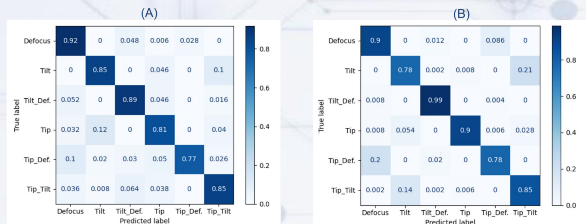
Top: Training accuracy and loss curves Bottom: (A) Confusion matrix for one test set - Test accuracy: 85%, (B) Confusion matrix for second test set - Test accuracy: 87%
