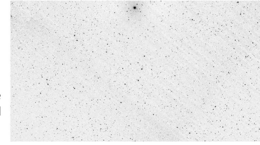
$\leftarrow$  Zoom-in (**2.3deg x 1.3deg**) of a NEOSTEL image taken at Turate site. The channels (3 visible here) of the FlyEye provide a uniform FoV.
