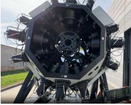
The FlyEye allows the survey of two-thirds of the visible sky three times per **night** revolutionizing **time-domain astronomy**, enabling comprehensive studies of transient phenomena and placing FlyEye in a new era of exploration of the dynamic universe. Efforts to develop automated calibration and testing
