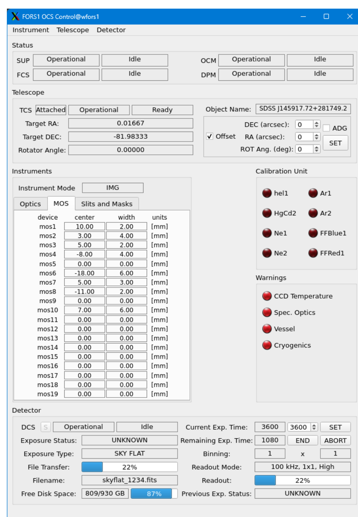
The first version of the FORS1 OCS Control GUI, designed to monitor the status of the instrument during regular science operations.
