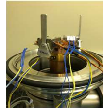
Figure 1: Lifetime test configuration of the FM of the Shutter
