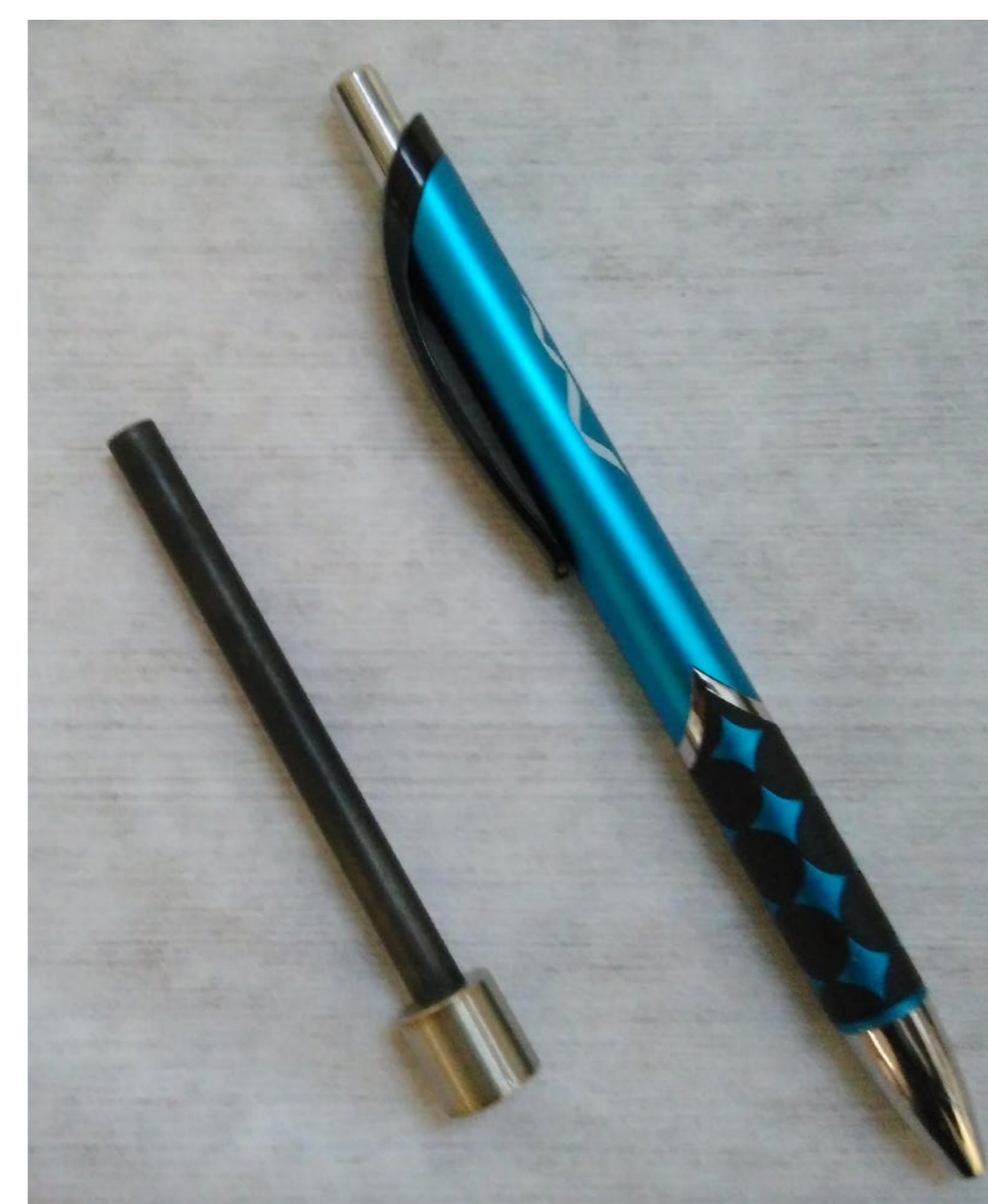
Fig. 3: Li scatterer encapsulated in a Be cylinder.
